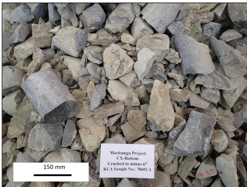
Figure 13-7: Fenix South Lower Sample Crushed to Minus 150 mm
